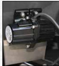
Prewired for Optional Vibrator Kit Shown Installed (3020340)
