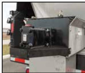
High Torque Auger Motor
