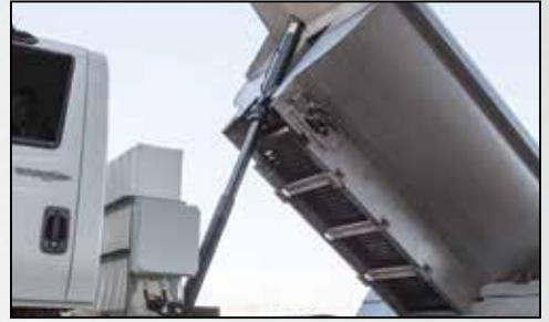
designed with a 3-stage, double-acting, front trunnion-mounted hoist
