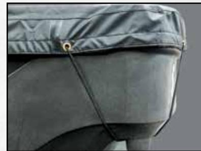
The fitted tarp has integral stretch cords with no "loose" parts to allow for fast installation.
