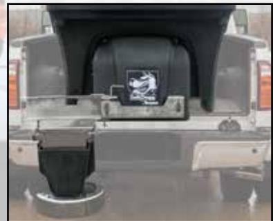
Swing-away chute for bulk unloading
