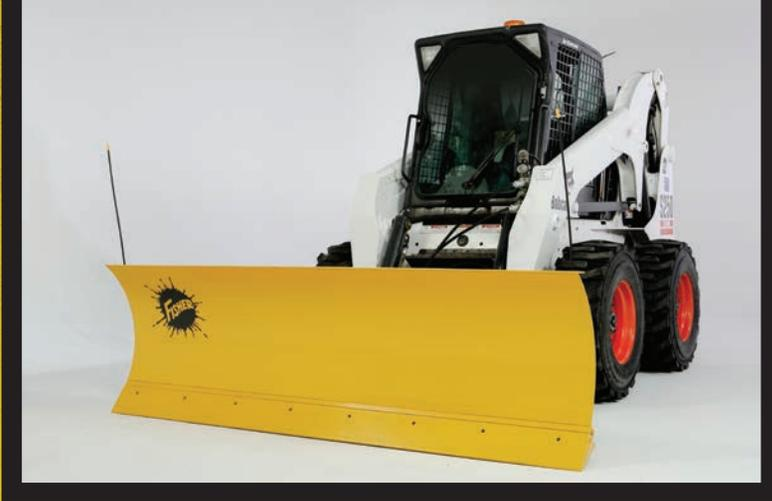
The rugged FISHER® **HD Series** snowplows withstand the rigors of commercial plowing. Available in 7'6", 8', 8'6" and 9' widths, the HD Series has been the choice of plowing professionals for many years.
