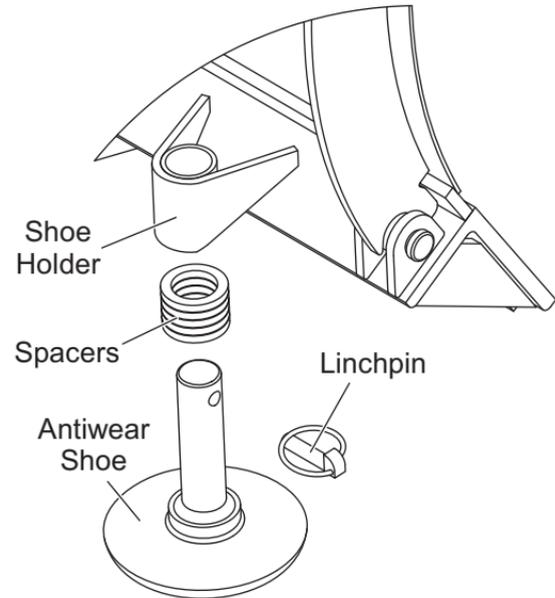
Standard shoe kit shown. An optional shoe kit, available for the HT Series™ and SD series blades, has a bolt-on shoe holder.
