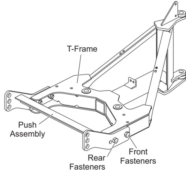
5. Select the hole in the rear of the T-frame that is best aligned with the rear hole in the push assembly and reinstall the rear fasteners. Tighten all four fasteners to 250 ft-lb.
