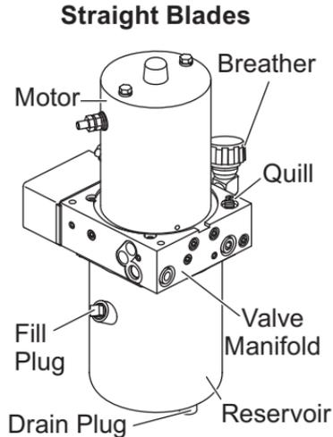
The HT Series™ hydraulic unit has blade scrape lock circuitry built into it. This feature resists the tendency a snowplow has to "float up" as larger amounts of snow build up in front of it while plowing deep snow, or stacking snow into piles. This feature is activated when the blade is in FLOAT, and is factory set. See your sales outlet for adjustment. The HT Series blade is raised in approximately 4 seconds and angled side to side in approximately 3 seconds.
