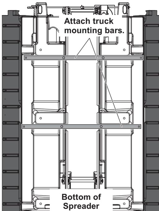
4. The spreader can be moved into the truck bed either by lifting the spreader by the four molded-in handles located on the corner legs or by sliding the spreader into the truck bed from the ground.
