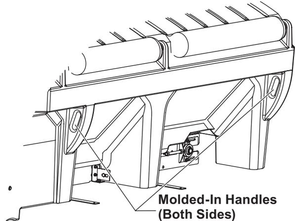
5. To lift the spreader into the truck bed from the ground, stand the spreader up on the feet at the rear of the spreader on top of two spacers at least 2" off the ground. The chute must be removed.
