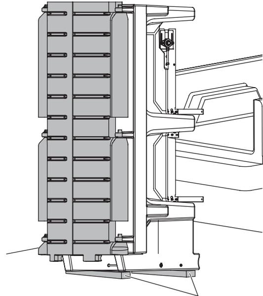
7. **Do not leave an unsecured spreader standing on its feet.** After pulling the truck away, either lower the spreader so it is resting on its six legs or properly support it with blocks and secure it as directed under "Storage" in the Maintenance section of this manual. If lowering the spreader onto its 6 legs, place spacers under the legs so the feet at the rear of the spreader are off the ground.
