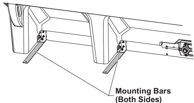
**NOTE: Pay special attention when drilling or clamping dissimilar metals to aluminum bodies. Galvanic corrosion can occur if not handled properly. Contact vehicle manufacturer for recommended attachment practices.**
