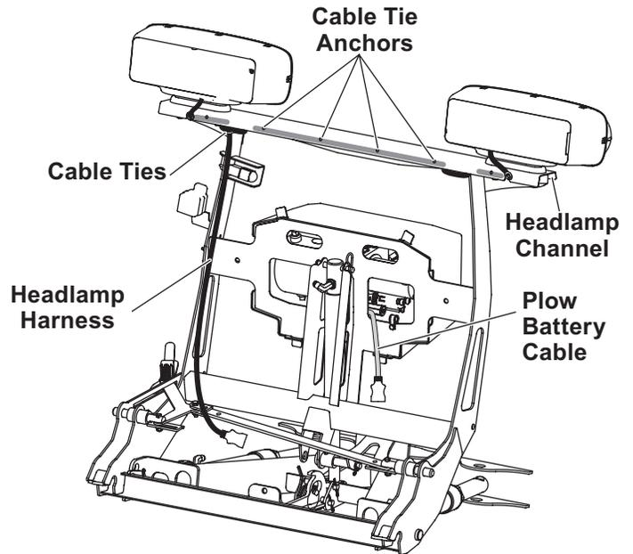
5. Cable tie the harness to the headgear as shown in illustration.
