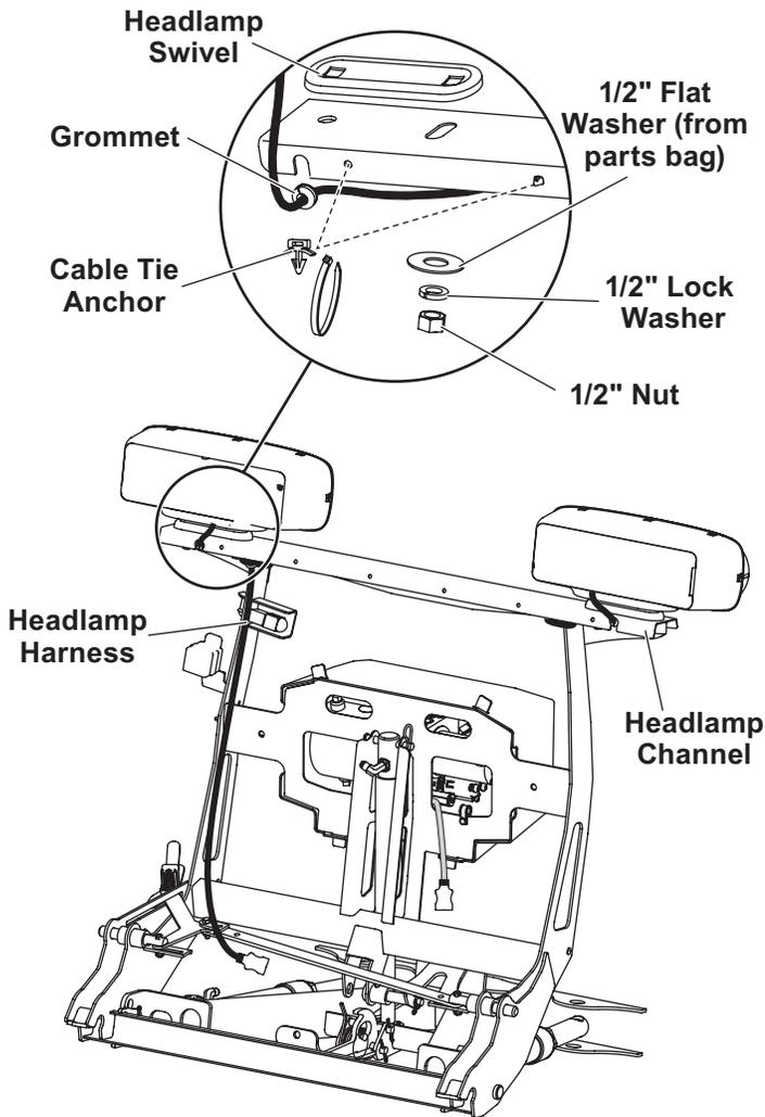
2. Insert cable tie anchors into the 1/4" holes on the rear of the headlamp channel, from inside the channel, with the locking tabs horizontal.
