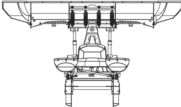
1. Fully angle the blade to one side. Lower the blade and turn the plow control and vehicle ignition OFF.
