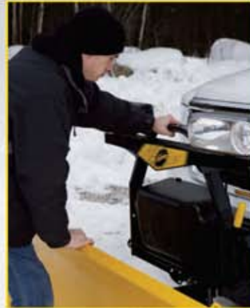
The proven Minute Mount® 2 System is simple, reliable and fast. The new HT Series snowplow features a handy push-bar that makes mounting even easier. It also features multiplexed electrical technology.
