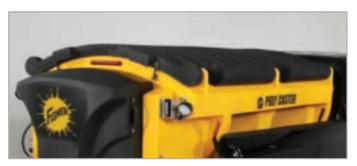
The overlapping poly hopper covers shield de-icing material from the elements. Its overlapping design seals out moisture while molded water grooves direct runoff away from hopper. Its domed shape increases hopper capacity. In the open position, the covers act as spill guards and protect the truck from material overflow while loading.
