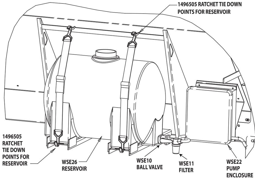
**Fig. 2 Reservoir Ratchet Tie-Down Pump Enclosure Installation**
