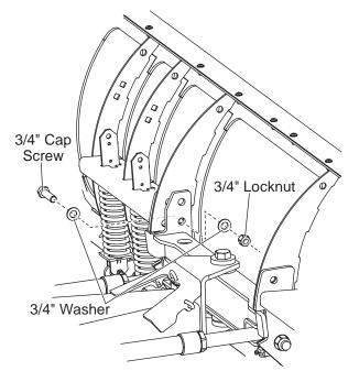
4. Torque upper and lower fasteners as shown:
