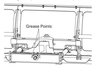
Grease the pivot beam at the beginning of the snowplow season. Reapply as needed during the season and before putting the snowplow in storage.
