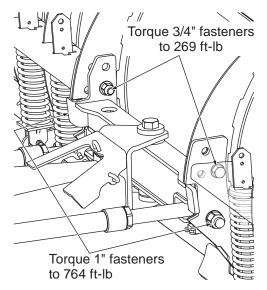
NOTE: Lower 1" locknuts must be torqued to 764 ft-lb, and the upper 3/4" locknuts must be torqued to 269 ft-lb.
