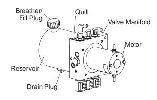
The Insta-Act® hydraulic unit's angling gives you full control of the snowplow from within the cab. Hydraulic rams hold the blade at a desired angle. In XtremeV<sup>TM</sup>, XV2<sup>TM</sup>, and XLS<sup>TM</sup> blades, the rams operate each wing independently or together as a single unit. The XtremeV and XV2 blades are raised in approximately 2 seconds and angled side to side in approximately 2 seconds.
