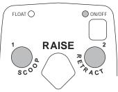
The two round buttons located to the left and right of the RAISE button move both wings at the same time into the blade positions described in the following table.
