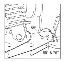
A special spring removal tool (20043) must be used to safely make this adjustment. NEVER ATTEMPT SPRING REMOVAL WITHOUT THE SPECIAL TOOL. Follow the instructions in the spring tool kit for proper tool usage.
