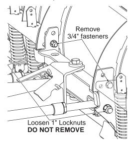
2. Align the desired attack angle holes in the quadrant and blade as shown.
