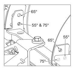
3. Reinstall the upper quadrant fasteners on both sides of the quadrant as shown.
