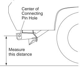
Find the appropriate range for your attack angle setting, and verify that the headgear is connected to the corresponding A-frame hole.
