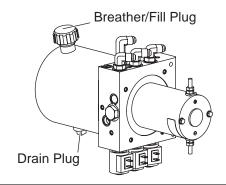
HT Series™ Blades: Fill the reservoir to within 2-1/2" from the top of the fill hole and replace the fill plug. For fluid recommendations see "Annual Fluid Change" in this section.
