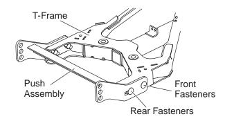
Select the hole in the rear of the T-frame that is best aligned with the rear hole in the push assembly and reinstall the rear fasteners. Tighten all four fasteners to 250 ft-lb.
