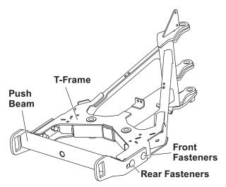
Select the hole in the rear of the T-frame that is aligned closest to the rear hole in the pushbeam. Lubricate and reassemble the previously removed fasteners into the rear holes. Tighten the fasteners according to the torque chart.
