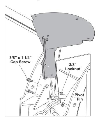
8. Install the blade guides with 5/16" x 1" cap screws and 5/16" locknuts, as shown.
