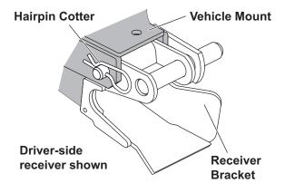
Measure the distance "d" from the ground to the top edge of the receiver bracket. Measure both sides and determine average value for "d."
