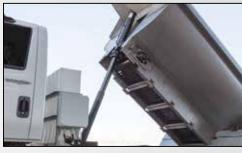
designed with a 3-stage, double-acting, front trunnion-mounted hoist
