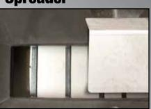
12" wide all steel pintle chain conveyor with stainless steel trough
