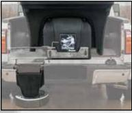
Swing-away chute for bulk unloading
