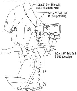
**5.** Insert **ONE** ½"**X2" HEX HEAD BOLT** (8) with **ONE** ½" **FLAT WASHER** (10) through the slotted holed towards the rear of the frame that aligns with the existing hole in the mount bracket. Secure with **ONE** ½" **LOCK NUT** (5).
